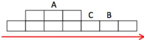
Fig. 3. Dangers of attaching blocks indiscriminately (side view of linear structure). If a robot at A adds a block to its left, it creates an unclimbable cliff; if it adds a block to its right, it creates an undescendable cliff. If a robot adds a block at B, it becomes impossible to add another at C.
