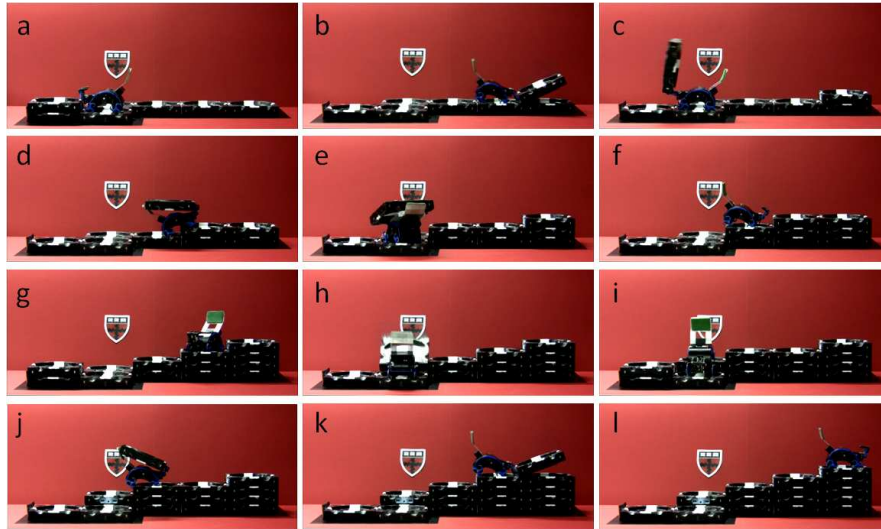
Fig. 13 Snapshots of a climbing robot building a 10-block 3D structure, collecting new blocks from a (manually reloaded) station at left.
