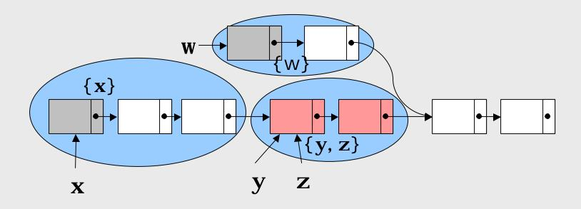
A location h is owned by a set of stack pointers S, if all paths from a stack pointer to the location h must go through the root of S
