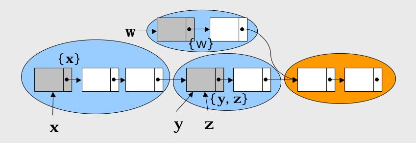
A location h is owned by a set of stack pointers S, if all paths from a stack pointer to the location h must go through the root of S
