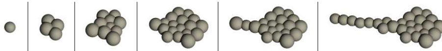
Fig. 1. Snapshots during the growth of a rounded structure with a narrow projection, grown using the model and approach for engineered morphogenesis described here.
