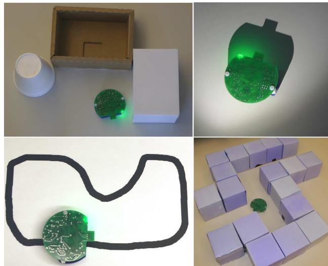
Fig. 1. Examples of behaviors the AERobot can be programmed to perform. Clockwise from bottom left: line-following, wall-following, phototaxis, maze-solving.
