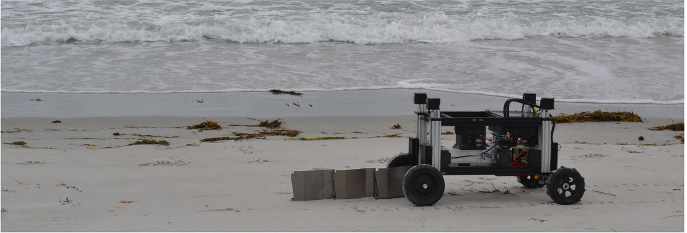
Fig. 1. Vision for Romu operating in a natural setting. Having installed the three piles it carries in one payload as the start of an erosion barrier, it heads for a supply cache to reload.
