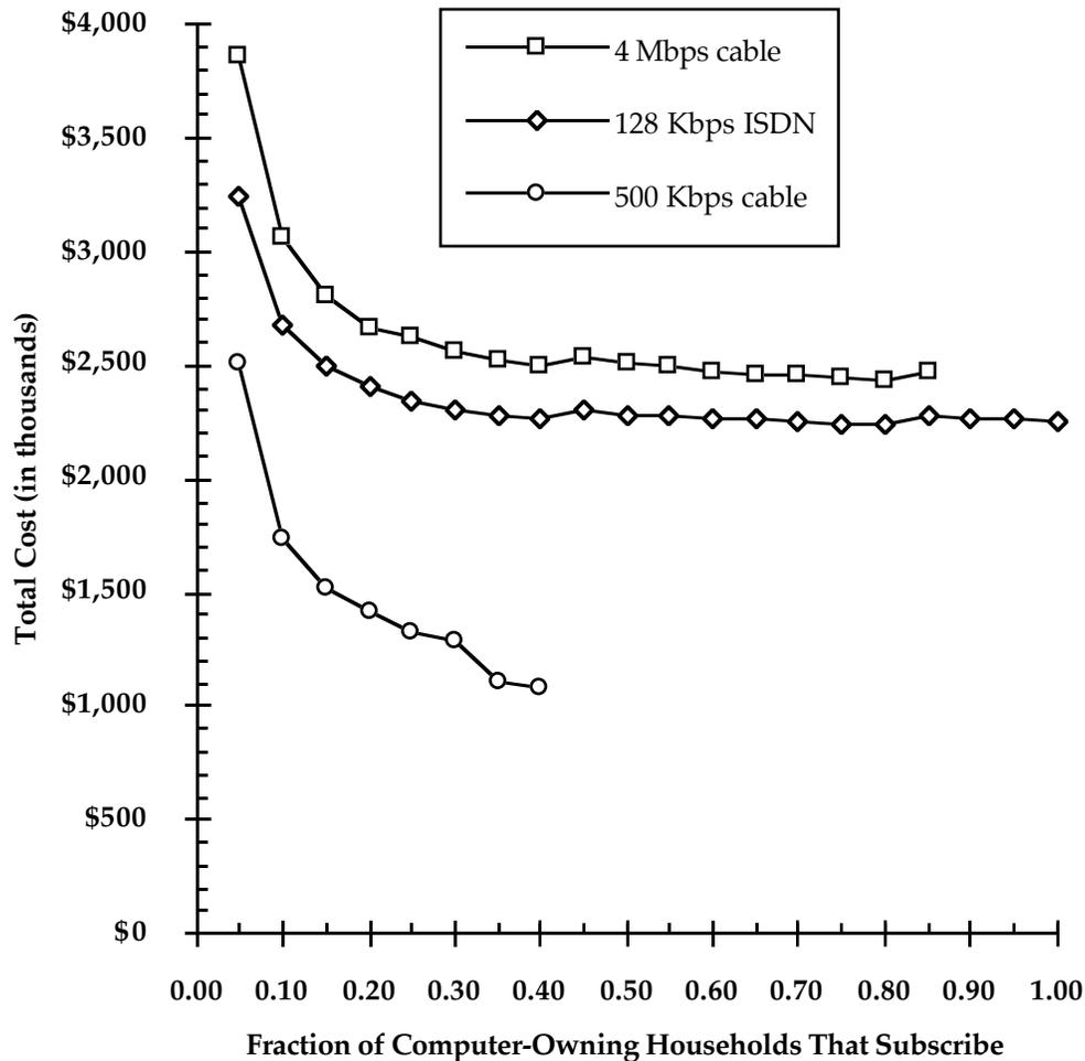
**Figure 7.16: Average cost with 30% of subscribers simultaneously active**
