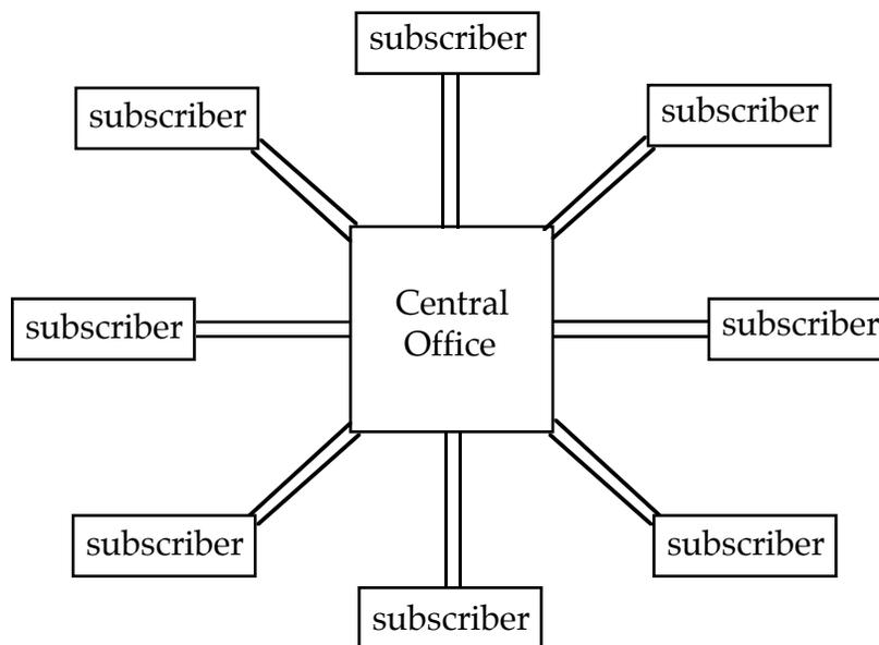
**Figure 4.2: Logical star architecture of local telephone network**
