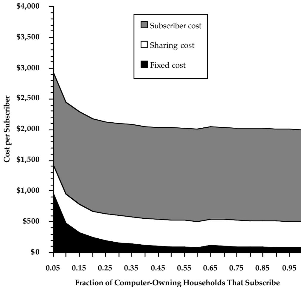
Figure 7.7: Components of average cost, 128 Kbps ISDN
