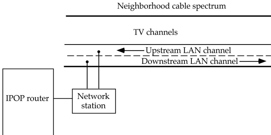
**Figure 3.8: Head end router connection to cable LAN**
