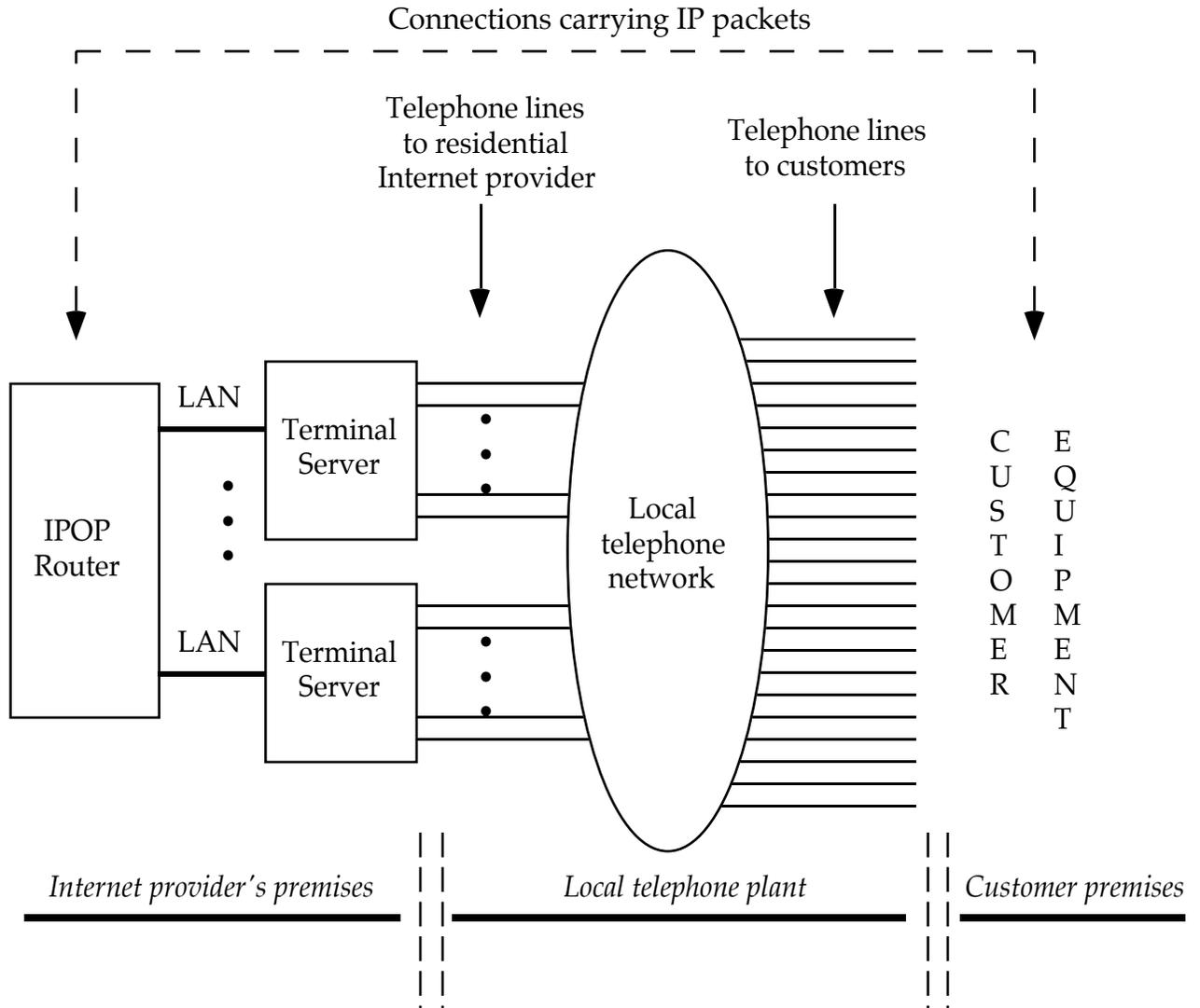
**Figure 4.8: Detailed view of point-to-point Internet access**
