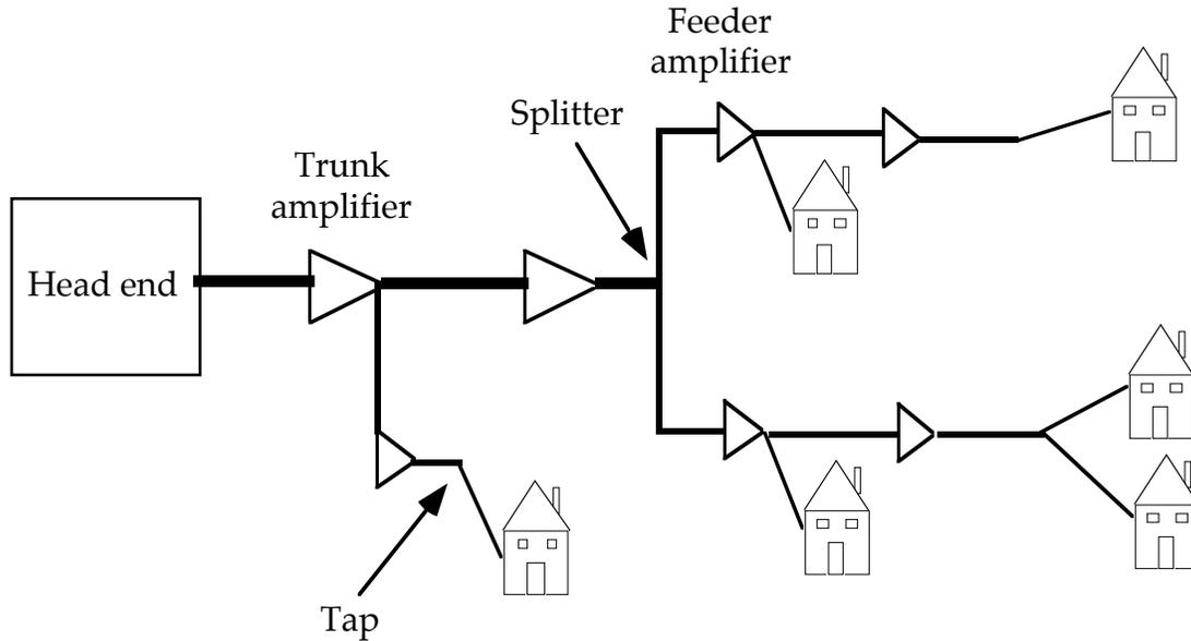
**Figure 3.1: Coaxial cable tree-and-branch topology<sup>40</sup>**
