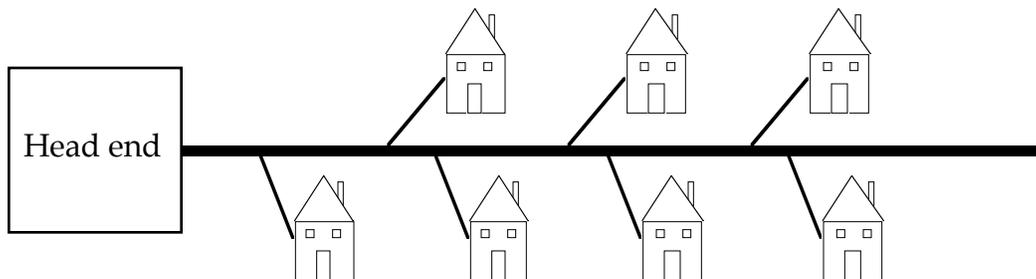
**Figure 3.2: Logical bus architecture of cable TV network**
