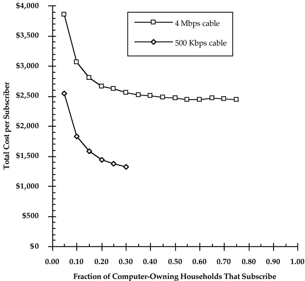
**Figure 7.20: Average cost with 60% cable LAN efficiency**
