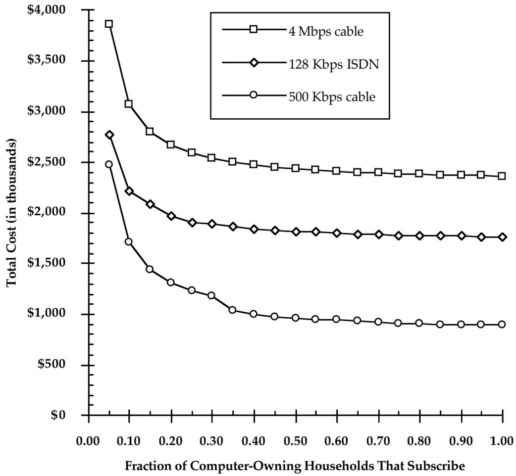
Figure 7.15: Average cost with 10% of subscribers simultaneously active
