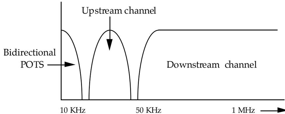
**Figure 4.6: Spectrum allocation for ADSL transmission<sup>92</sup>**
