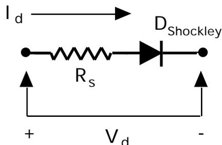
Using two data points, you should be able to determine both  $R_s$  and  $I_s$  for the actual diode -- 100 $\mu$ A and 10mA are two good current values to use for this type of diode. The following equation describes the model above:
