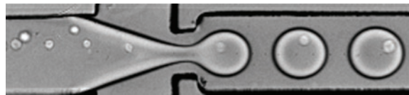
Figure 1 | Creation of water droplets containing single living cells inside a microfluidic device. Image courtesy of Christoph Merten.
