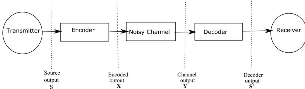
**Figure 2:** Block diagram with encoder and decoder
