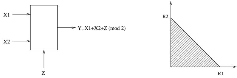
**Figure 4:** Binary Symmetric MA Channel
