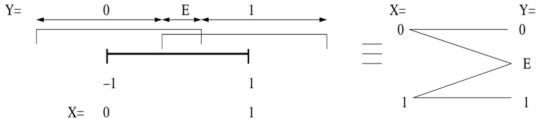
**Figure 1:** Model channel as a Discrete Binary Erasure Channel.
