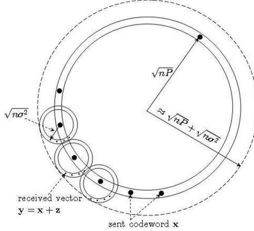
**Figure 3:** Sphere packing for the AWGN channel
