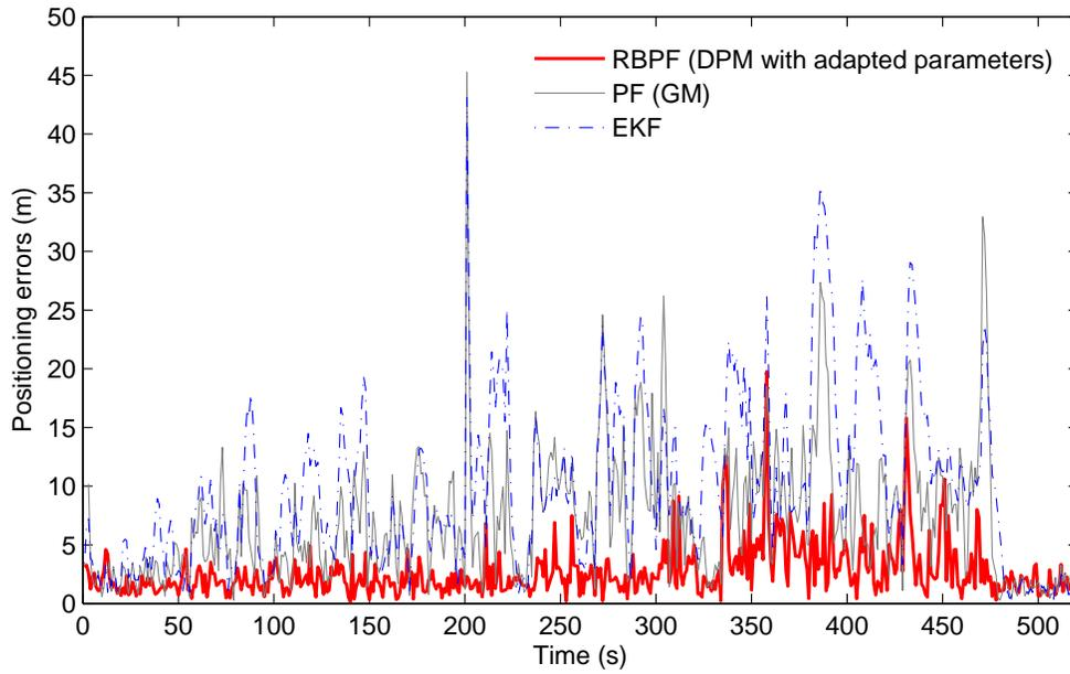
Figure 3: Localization error in Toulouse for the three methods implemented : DPM based method (red) overperforms the two others (blue = EKF and grey = particle filter).
