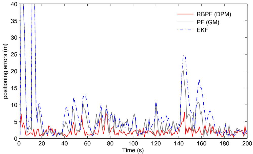
Figure 4: Localization error in Rouen for the three methods implemented : DPM based method (red) overperforms the two others (blue = EKF and grey = particle filter).
