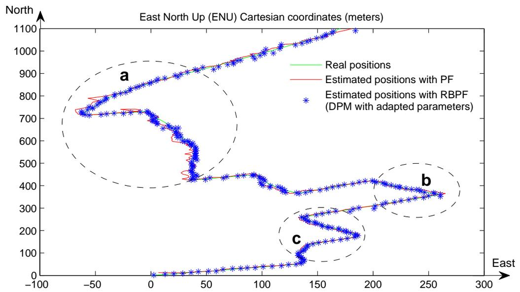
Figure 5: Real trajectory in Toulouse (green) and estimated trajectories : blue = DPM based method and red = particle filter based method
