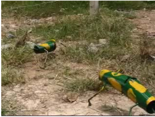
Figure 2: Legged robot that can walk freely on rough terrain and push a sledge to carry metal detectors
