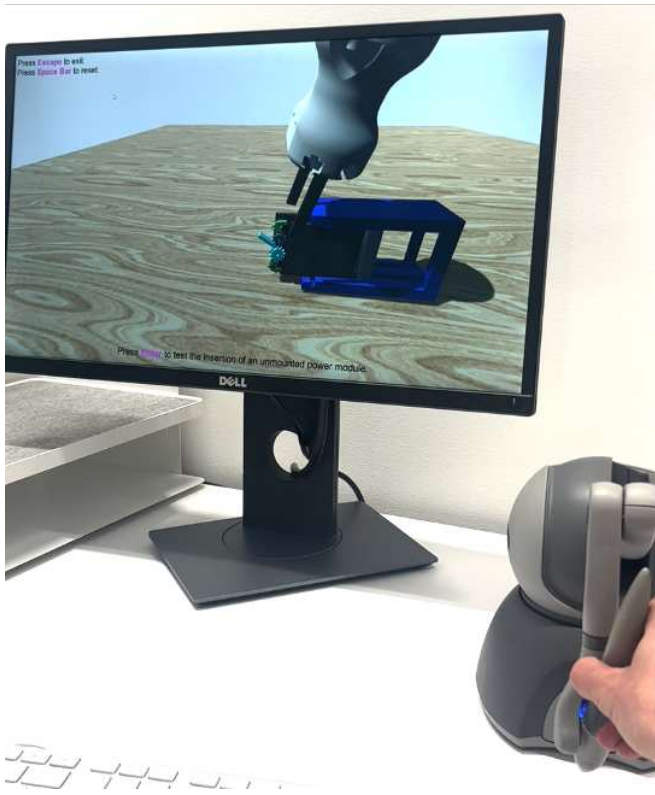
Fig. 1. A user interacting with our haptic design tool. A Phantom Omni / Geomagic Touch haptic device directly controls the pose and actuation of a simulated parallel-jaw gripper. The device provides force feedback reflecting collisions in a physics-based simulation. By playing the role of a robot attempting to operate some item of equipment in simulation, the user can better evaluate what the physical usability of that equipment would be for a robot, and identify points of particular difficulty. Incorporating such a tool into the design cycle can thereby facilitate designing equipment operable by autonomous robots, without requiring accurate intuition built on extensive robot experience.
